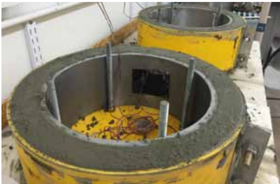
ASTM C1581: Restrained Ring Test (Days to Cracking)
